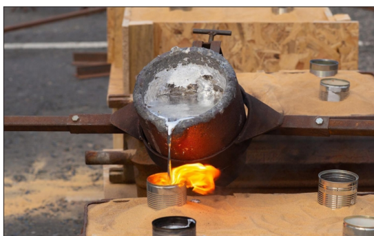
Molten metal was poured into moulds.
